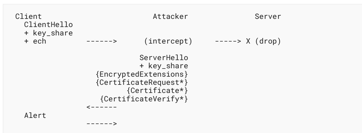
Figure 3: Client Reaction Attack
